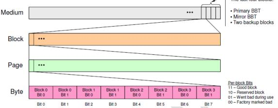
It marks as "Bbt0" in spare are of Primary BBT, and marks as "1tbB" in spare area of Mirror BBT.
